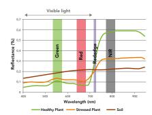
The health of crops can be identified depending on how they reflect light in the different wavelengths
